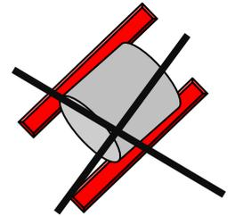
**2. NO INSTALARME SOBRE VIGAS O PERFILES. EL DEPOSITO ENTERO INCLUIDAS LAS PATAS DEBEN DESCANSAR EN LA BASE.**
